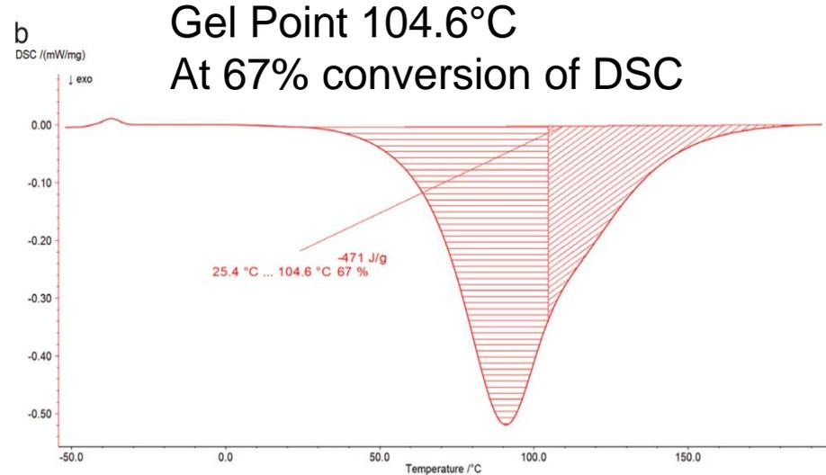
b) Heat flow measured during the temperature ramp at 3 K min<sup>-1</sup>
