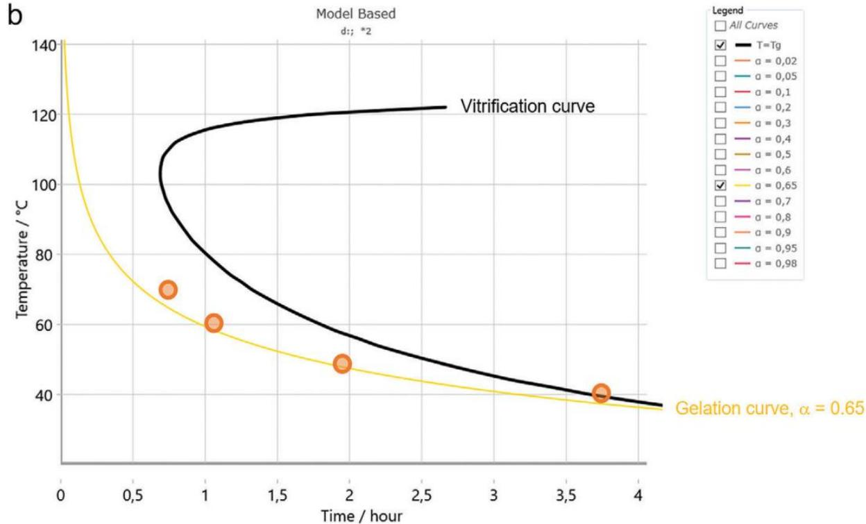
b) Prediction of the gelation curve (yellow) and measured gel point times at 40, 50, 60, and 70 °C (orange circles)
