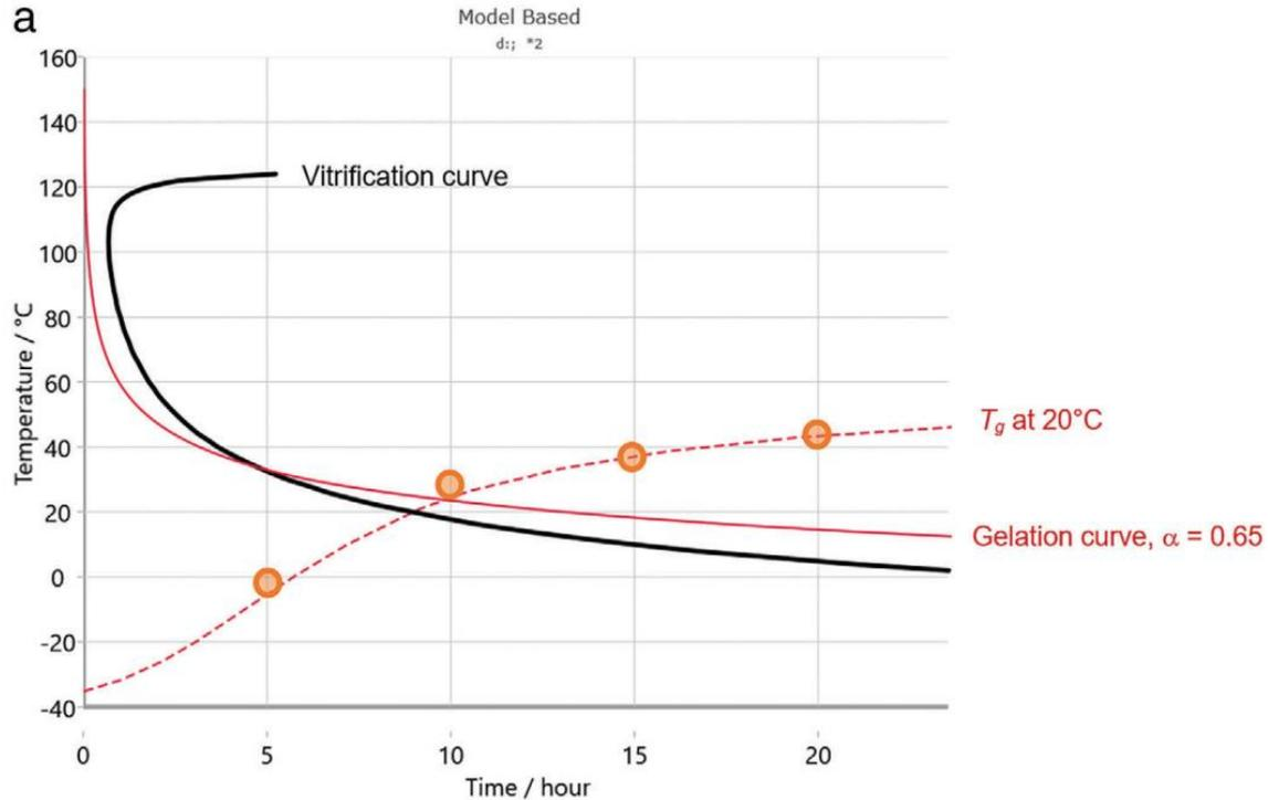
a) Prediction of the glass transition temperature (dashed, red) and measured glass transition temperatures (orange circles) after 5, 10, 15, and 20 h at 20 °C
