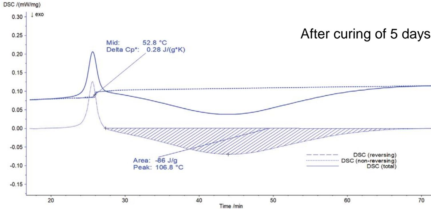
Total, reversing, and nonreversing heat flows of a mixture cured at room temperature during the course of five days
