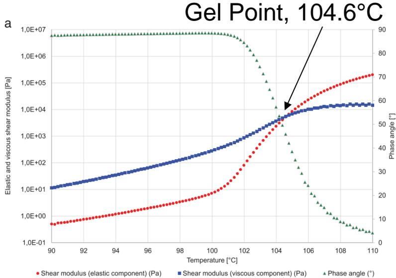
a) Elastic and viscous shear moduli, phase angle measured during the temperature ramp at 3 K min<sup>-1</sup>
