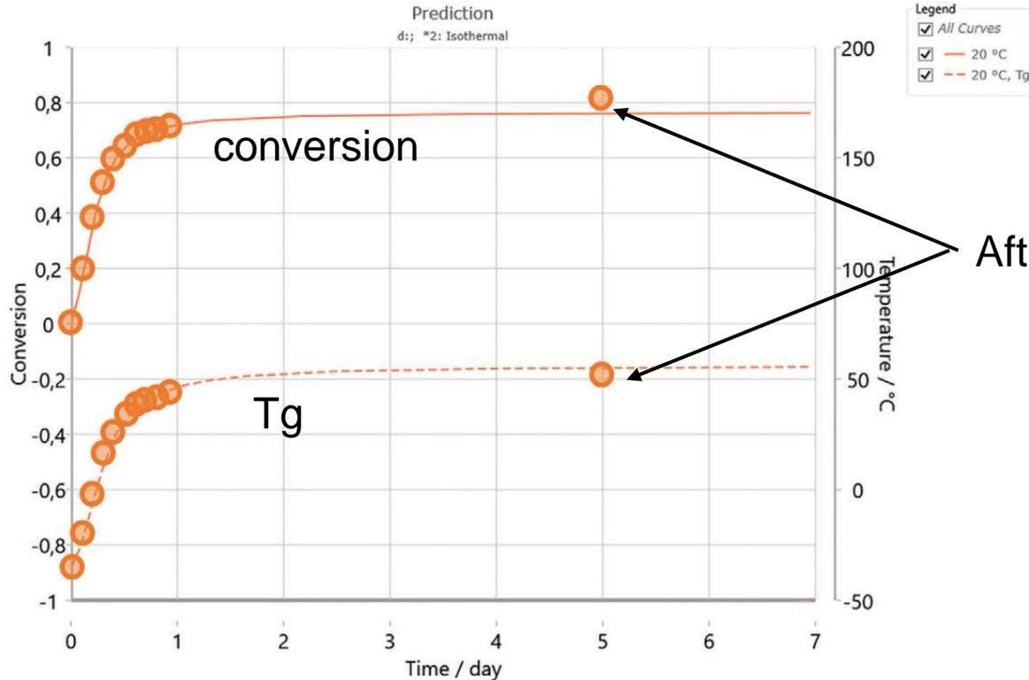
Prediction of Kinetics Neo for curing at room temperature
