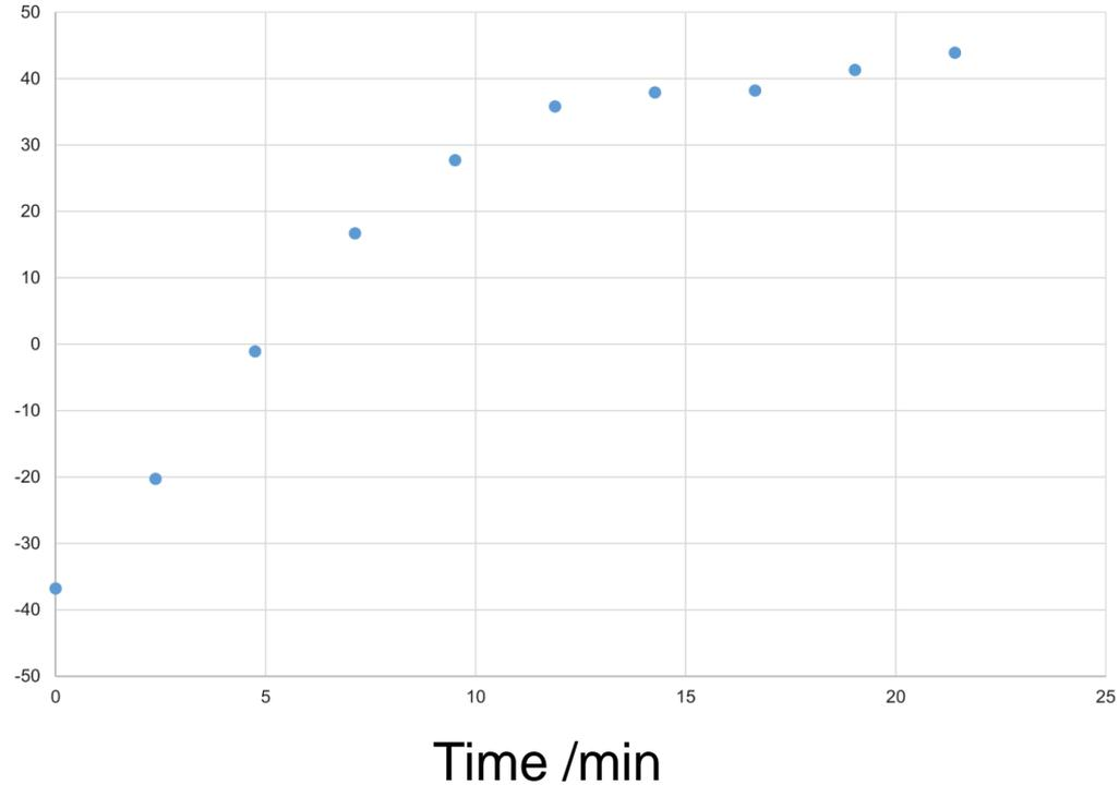
Progression of the glass transition temperature (midpoint) as a function of the curing time at 20 °C
