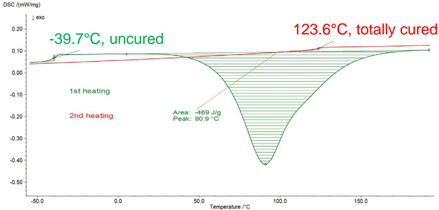
Total heat flow of the modulated DSC measurement performed on sample 1 during the first and second heating
