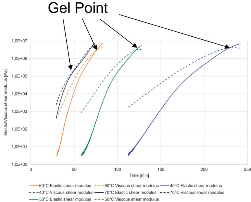
**Table 3.** Gel point time obtained for the different isothermal tests.
