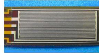
IDEX sensor for DEA cure monitoring
